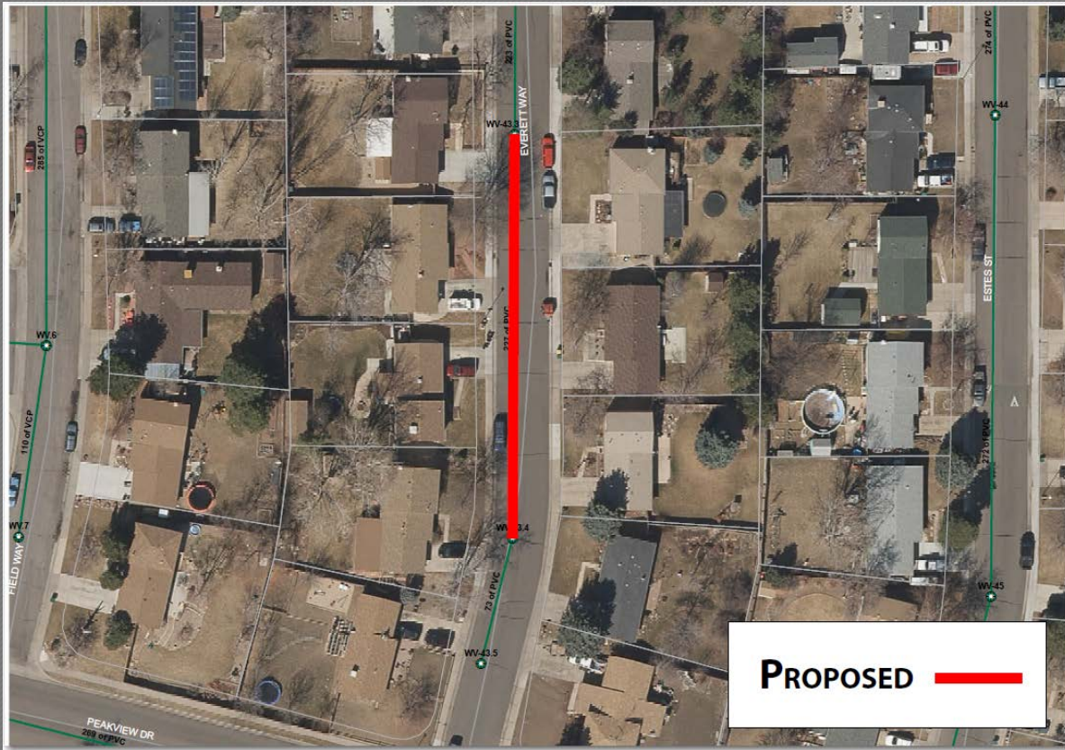
Everitt Way north of Peakview Dr Replace 227' of 8" Sewer main
