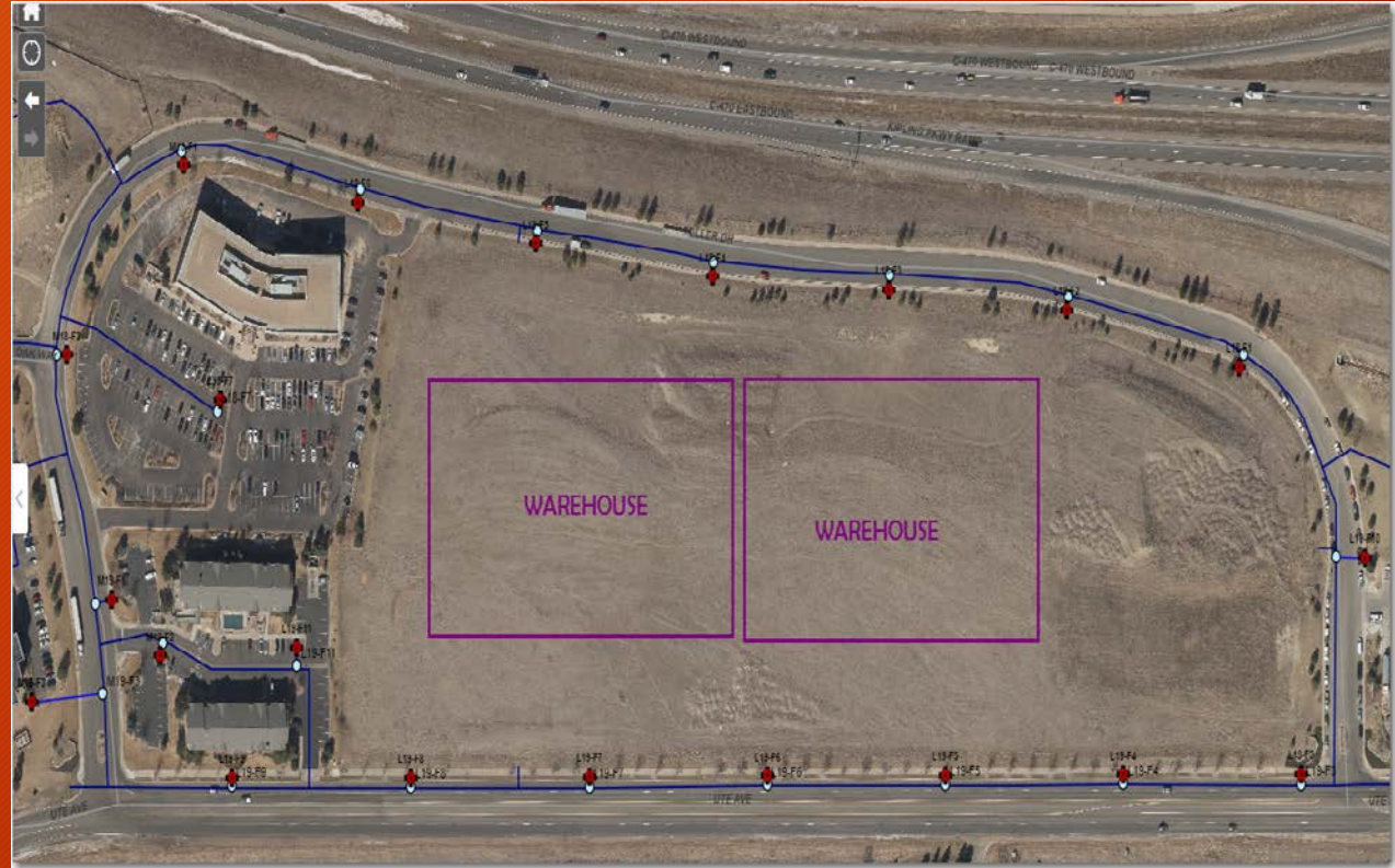
Existing Water Main and Hydrants
