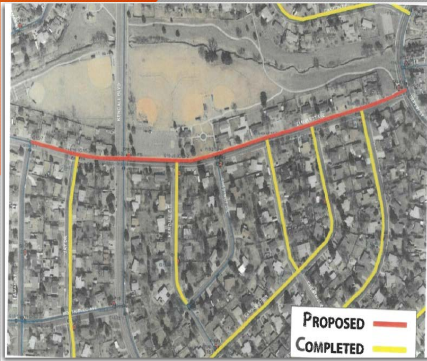
Elmhurst between Lamar and Depew – 2300' 12" PVC
