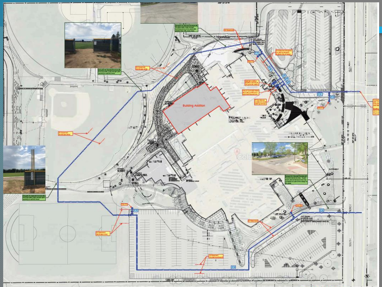
Original Water Pipe Configuration
